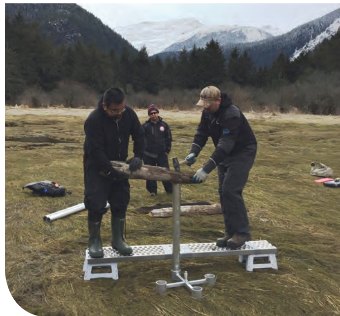
Members of the Nuxalk Guardian Watchmen install an instrument to measure sediment deposition in the Asseek Estuary located within the traditional territory of the Nuxalk First Nation, British Columbia./Karen Barry
